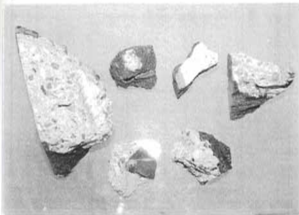
Figure 4.26 Monolithic behavior between existing concrete and replacing cement grout in specimen U-AT8-1
